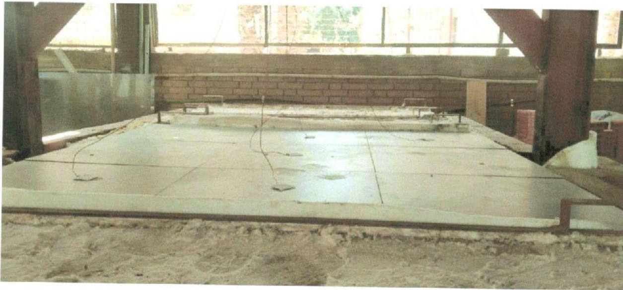
Figure (1): Un-exposed surface of tested assembly before the fire resistance test
